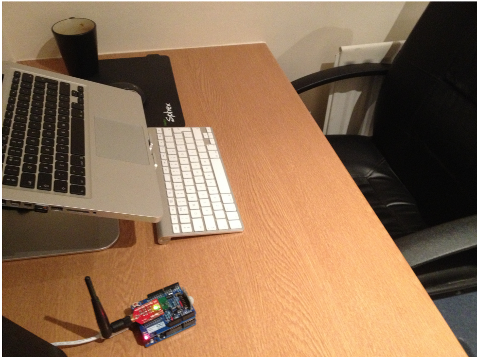
Figure 21: Typical deployment of the sensor node at a desk during the field trial
